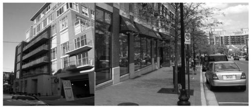
Access to below-grade parking should be located off side streets and lanes to reduce curb-cuts on Bloor Street West and Dundas Street West
